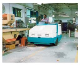
The brush and vacuum filter system combination makes the 6500 ideal for factory floors.
